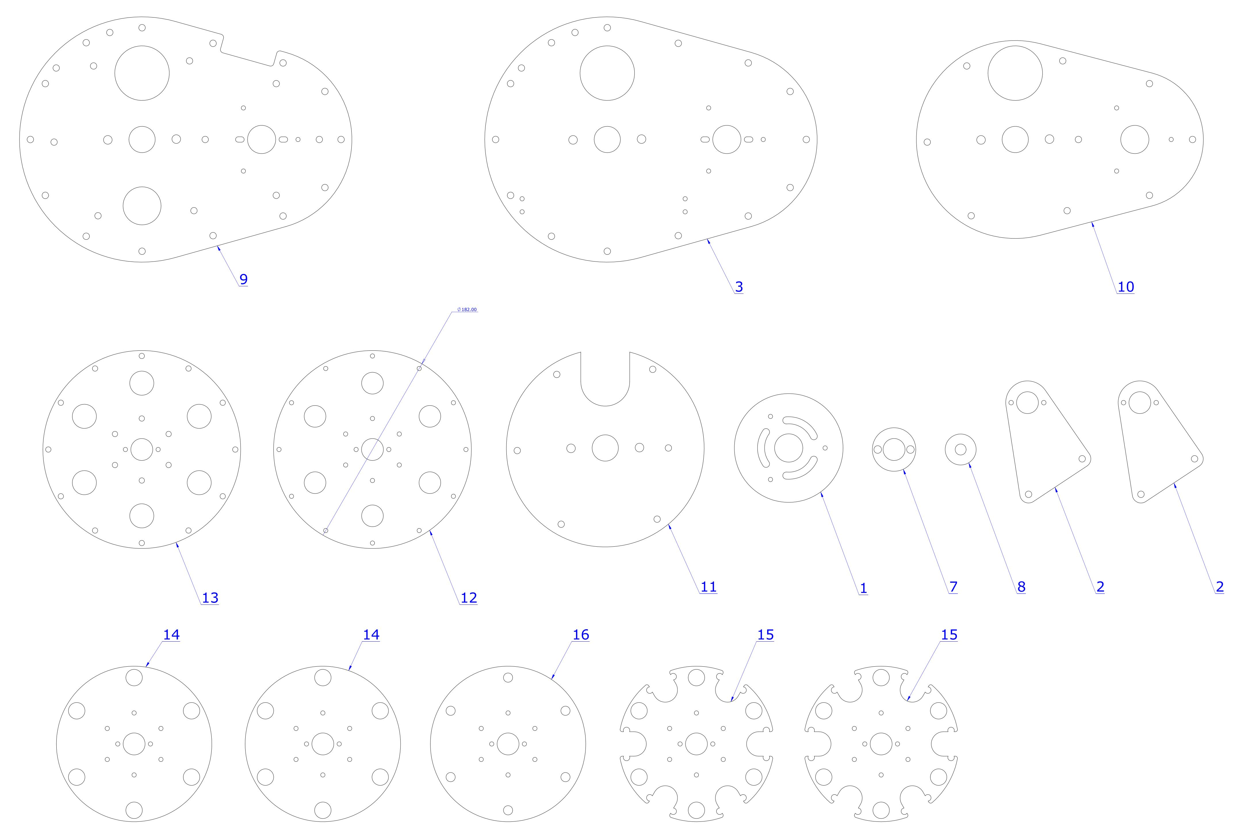
Scale 1:1 1 off of each part in 4mm Aluminium
